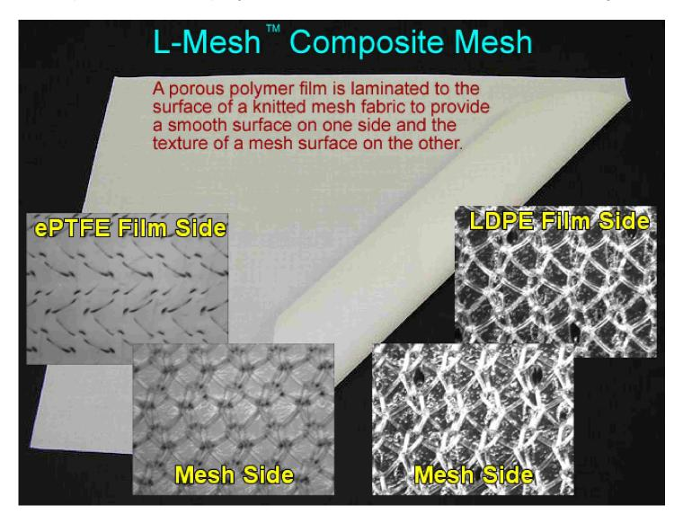
L-Mesh™ composite mesh is a laminate of knitted mesh and porous polymer film. Composite mesh fabrics are available with an expanded polytetrafluorethylene (PTFE) film surface or a porous low density polyethylene (LDPE) film. The result is a flexible and resilient sheet with a mesh surface on one side and a smooth porous film on the other side.
